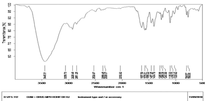
Figure 5. FTIR of HPMC-K 15
