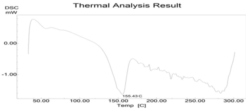
**Figure 8.** DSC analysis of HPMC-K15
