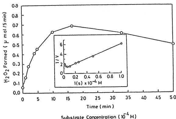
Fig. 4. Dependence of initial velocity of purified oxalate oxidase reaction on substrate concentration. Standard assay conditions were used for the incubation period, which was varied as indicated. The inset shows the double reciprocal plot for oxalate. All points were derived from Fig. 4.
