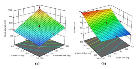
Figure 2. Response surface plots showing the combined effect of the amount of nanocellulose and PEG on (a) tensile strength and (b) % release.
