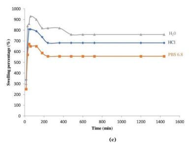
Figure 3. Swelling property of (a) XF (b) NF, and (c) XNF in distilled water, HCl, and phosphate buffer
