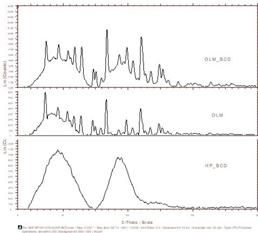
**Figure 4.** X-ray diffraction patterns of Pure Olmesartan Medoxomil (OLM), Hydroxypropyl  $\beta$  cyclodextrin (HP  $\beta$ CD) and kneading complex of Hydroxypropyl  $\beta$  cyclodextrin (HP  $\beta$ CD) and Olmesartan Medoxomil (OLM)
