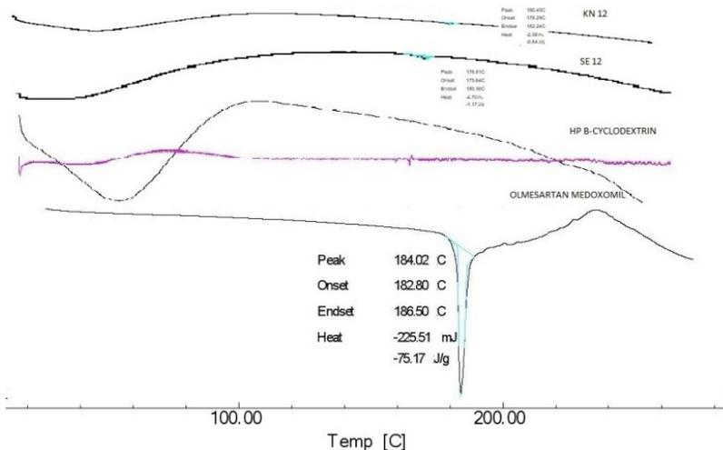
**Figure 2.** DSC curves of Pure Olmesartan Medoxomil (OLM), Hydroxypropyl  $\beta$  cyclodextrin (HP  $\beta$ CD), Olmesartan Medoxomil (OLM): Hydroxypropyl  $\beta$  cyclodextrin (HP  $\beta$ CD) kneaded complex (1:2), and Olmesartan Medoxomil (OLM): Hydroxypropyl  $\beta$  cyclodextrin (HP  $\beta$ CD) solvent evaporated complex (1:2).
