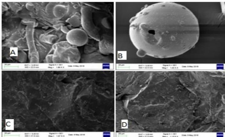
**Figure 3.** Scanning electron microscopic images of A- OLM and HP-  $\beta$  CD, B- HP-  $\beta$  CD, C -Inclusion complex of HP  $\beta$ -CD (SE 12) and D- Inclusion complex of HP  $\beta$ -CD (KN 12)
