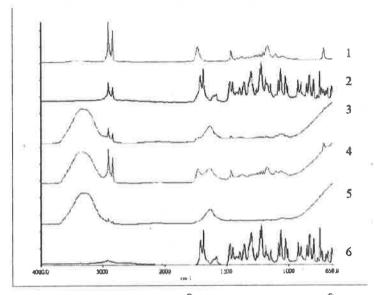
Figure 1. ATR-FTIR Spectra of Compritol<sup>®</sup> 888 ATO (1), Compritol<sup>®</sup> 888 ATO: indomethacin, Physical Mixture (2), solid lipid dispersion formulation F1 (3), F3 (4), F5 (5) and pure indomethacin (6).
