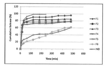
Figure 3. In vitro dissolution profiles of indomethacin loaded solid lipid microparticle formulations and indomethacin alone.
