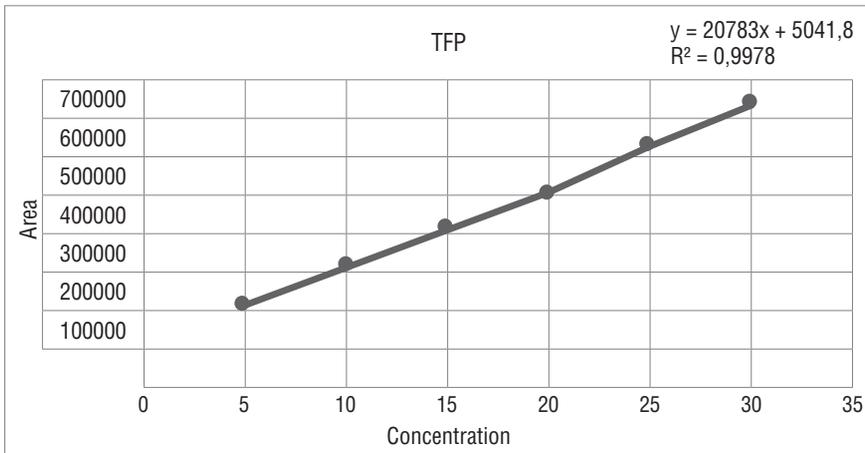
Figure 18. Calibration curve of TFP (5-30 µg/ml)
