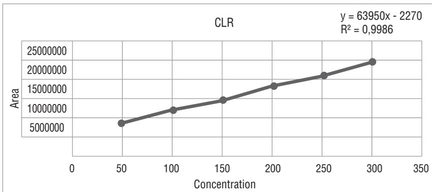
**Figure 19.** Calibration curve of CLR (50-300 µg/ml)
