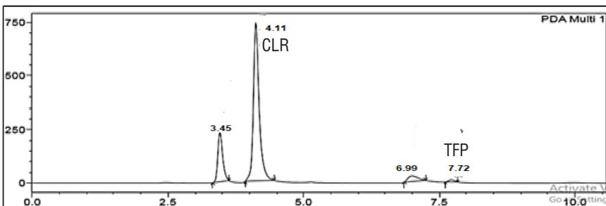
Figure 6. Chromatogram of photolytic degradation
