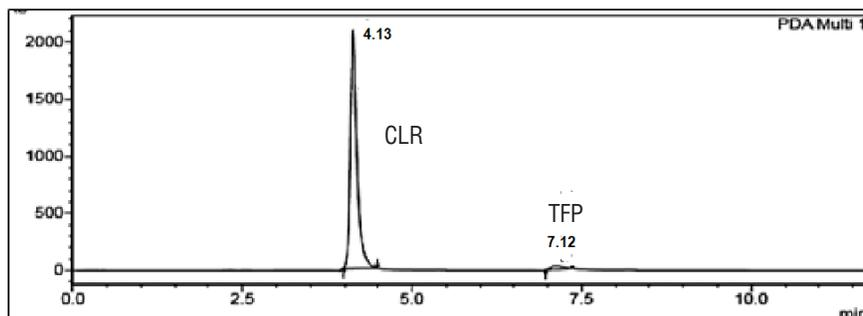
**Figure 10.** Standard chromatogram of CLR and TFP
