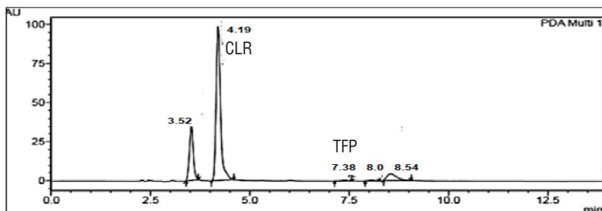
**Figure 7.** Chromatogram of oxidative degradation
