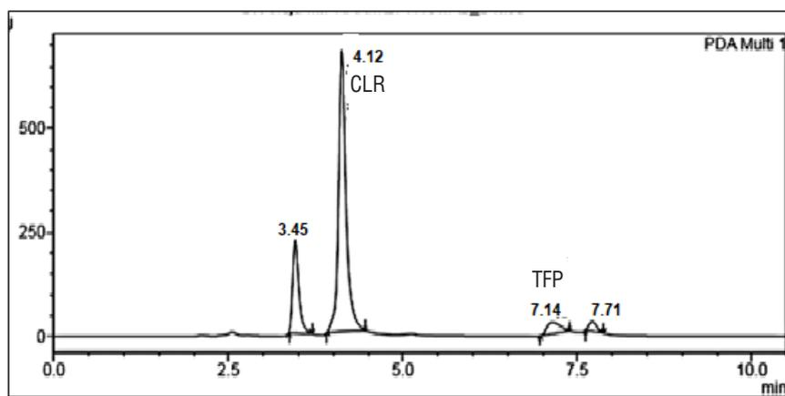
**Figure 9.** Chromatogram of neutral degradation
