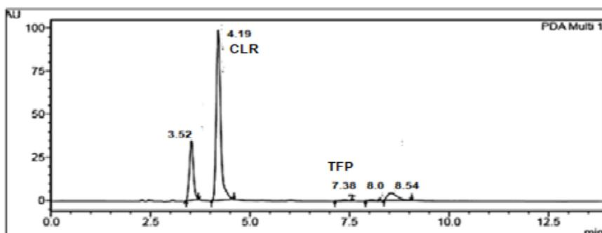
Figure 15. Specificity chromatogram (oxidative degradation)
