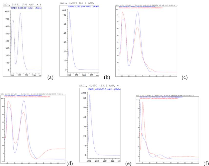
**Figure 3.** (a) UV spectra of M5 standard; (b) UV spectra of M1 standard; (c) Comparison of UV spectra from standard M5 and metabolically formed S1 test (22.010 min); (d) Comparison of UV spectra from standard M5 and metabolically formed M5 and S2 control with no co-factor (21.652 min); (e) M1 standard UV; (f) Comparison of UV spectra from standard M1 and metabolically formed S2 test (3.463 min); (d), (e), and (f) UV spectrum of S2 with pig microsomes fortified with NADPH
